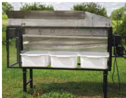
Breckel’s invention, the Ocooch Mountain Rotary Destemmer.
